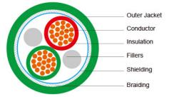
The series TORSION and FESTOON are used to interconnect Profibus BUS components. This BUS system is a very economical solution for the field area. For the information exchange between different automation systems as well as for communication with the connected decentralized field units, serial field bus systems are used. The lines described here are designed torsionable or hanging movable construction. Areas such as robot applications and/or garland suspension are easily realized.
