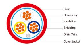
CC-Link® (Control & Communication Link) is a field network system that processes
